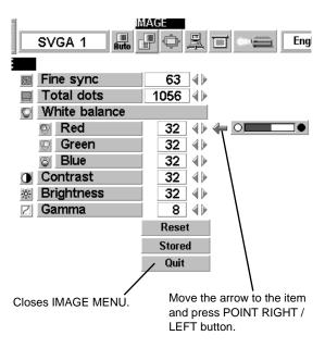
NOTE : The Fine sync and the Total dots cannot be fully adjusted when "RGB," "HDTV1035i" or "HDTV1080i" is selected on the SYSTEM MENU (P22 and 23).
