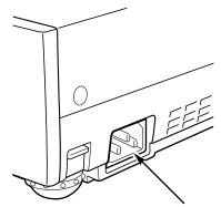
Connect the AC Power Cord (supplied) to the projector. The AC outlet must be near this equipment and must be easily accessible.
