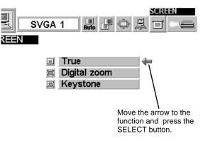
NOTE : The True and the Digital Zoom cannot be operated when "RGB," "HDTV1035i" or "HDTV1080i" is selected on the SYSTEM MENU (P22 and 23).
