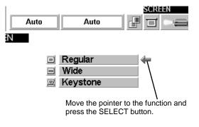
NOTE : The Regular and the Wide cannot be operated when "720p," "1035i" or "1080i" is selected on SYSTEM MENU (above).
